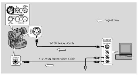
You cannot use headphones while doing analog line-in recording. If you have the AV/headphones terminal set to headphones, it will automatically switch to AV for analog line-in recording. PHONES disappears from the display.
